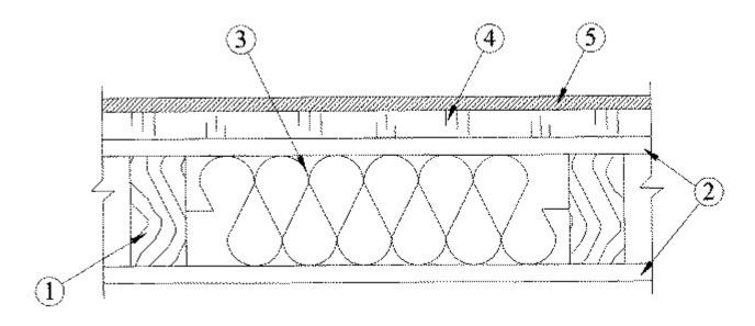
1. Wood Studs — Min. nom 2 by 4 in., spaced 16 in. OC.
