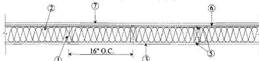
1. **Wood Studs** — Nom 2 by 4 in. spaced 16 in. O.C. Cross braced at midheight and effectively firestopped at top and bottom of wall.
