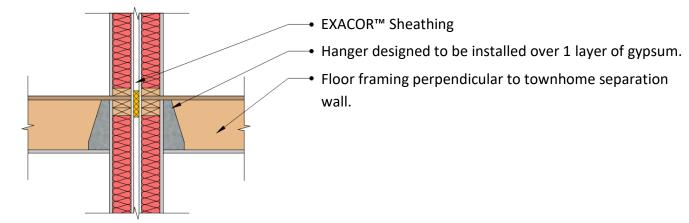
In this example, the wall framing is not interrupting the separation wall as the wall is continuous to the underside of the floor sheathing. The floor framing is supported by a joist hanger that is designed to be installed over 1 layer of 5/8" gypsum wallboard.
