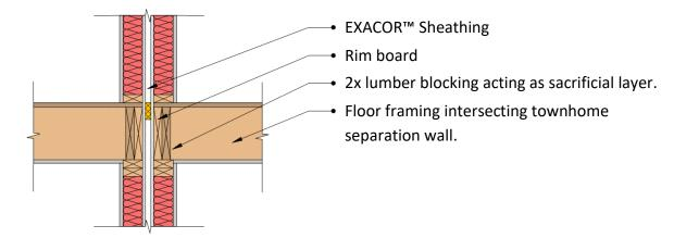
Chapter 16 of the NDS provides a nominal char rate of 1.5-inch/hour for solid sawn lumber. Therefore, installing a layer of nominal 2x lumber blocking to the rim board between the floor joists would provide 1-hr of protection to the rim board and continuity of the rated wall assembly.
