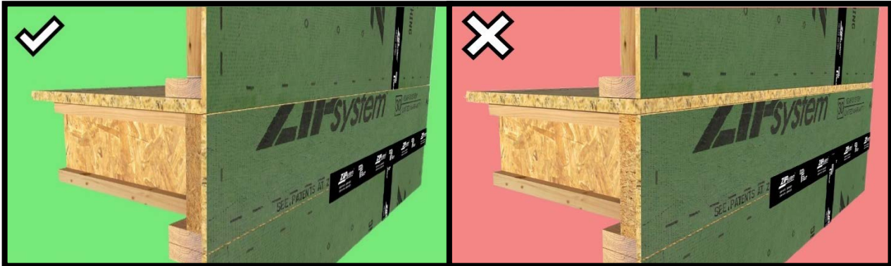
Figure 2: Plan ahead to ensure the ZIP System sheathing seam above the rim joist will take into account the thickness of the subfloor.
