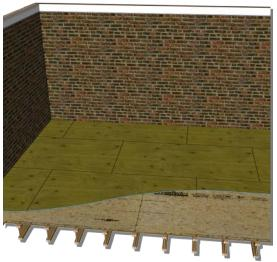
Fasten top layer using wood screws of sufficient length to just penetrate the thickness of the subfloor. <u>Do not</u> screw second layer to floor joists.
