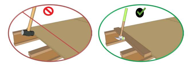
PRO TIP: Install the first row of AdvanTech X-Factor subflooring with the tongue profile oriented towards the exterior. This allows for the wooden block to be placed on the groove when tapping the panel into place. This prevents crushing of the tongue.
