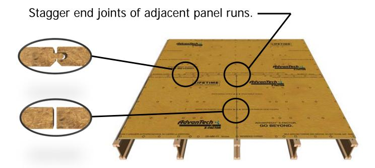
PRO TIP: use 10d nails to space the AdvanTech X-Factor subfloor panels 1/8-inch.
