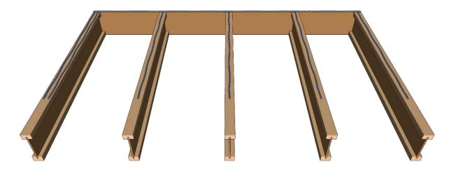
Immediately after applying the adhesive, lower the panel into place, making sure the panel is square on the joists. The top side of the panel should be facing up to allow for the certification stamp to be easily viewed from the bottom by local building officials. Panels should span two or more spans (three or more floor joists) with the long dimension perpendicular to the floor framing.
