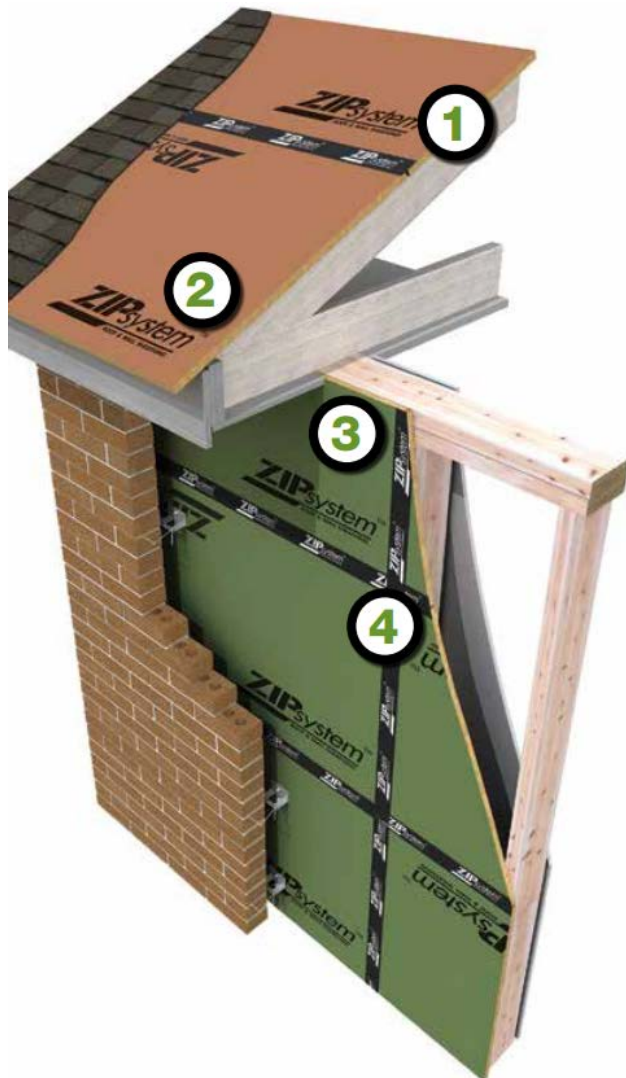
Figure 1: ZIP System Description and Integration into a Building
