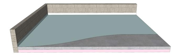
For both installation methods, the structure must be fully enclosed and dried-in prior to subfloor application. Do not install AdvanTech over a concrete slab while exposed to elements.
