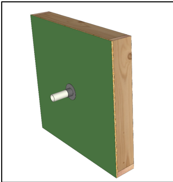
FIGURE 1 – TYPICAL FLASHING FOR THROUGH WALL PENETRATION
