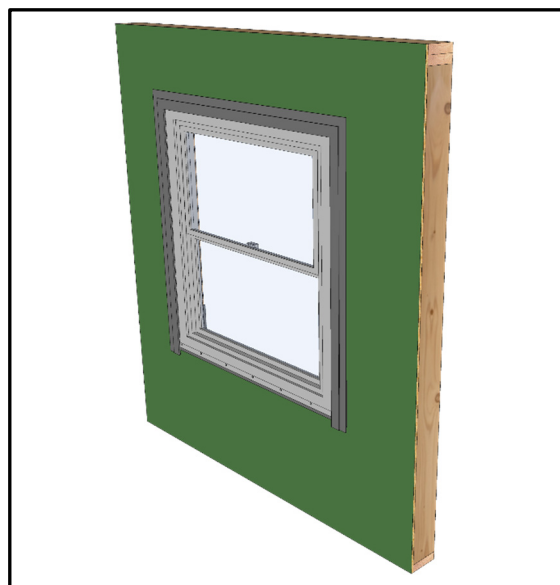
FIGURE 3 – TYPICAL FLASHING FOR WINDOW FLANGE
