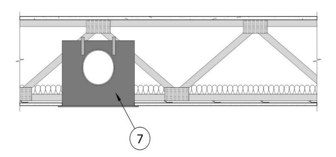
1. **Flooring System** — **Building Units\*** — Nom 3/4 in. thick. Long dimension of panels to be perpendicular to trusses with end joints staggered a min of 4 ft. and joints centered over the trusses. Panels secured to wood trusses with 2 in. x 0.113 in. Ring Shank nails spaced a max of 12 in. OC in the field and on the perimeter. Nails located 2 in. from panel corners, and 1/2 in. from panel edges. **HUBER ENGINEERED WOODS L L C**— Type 3/4 in. Shiplap Exacor™ Board
