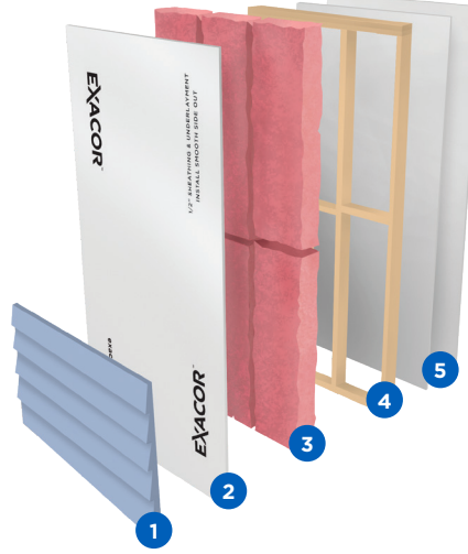
EXACOR MgO 2-HOUR WALL ASSEMBLY 1 MOS-1290-06 (ESL-1290)
